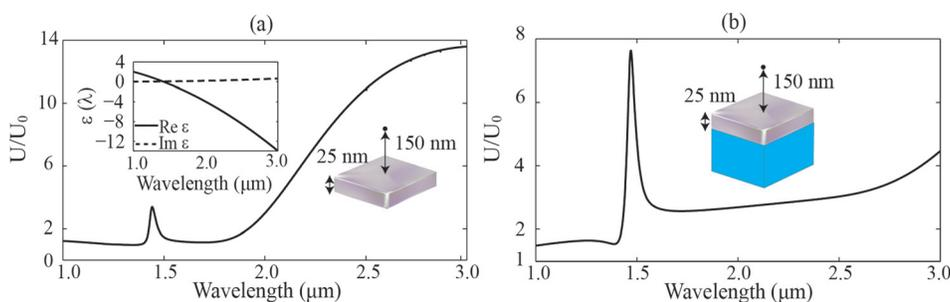
FIG. 2. (a) Normalized thermal emission for a 25 nm AZO slab; the observation distance is 150 nm. Coupled surface plasmons of thin films play a key role in the thermal emission. (b) Normalized thermal emission for a 25 nm AZO slab with a dielectric substrate ( $\epsilon=6$ ), the distance is 150 nm. The substrate leads to tuning of the SPP resonance and a narrowband peak in the thermal emission.
