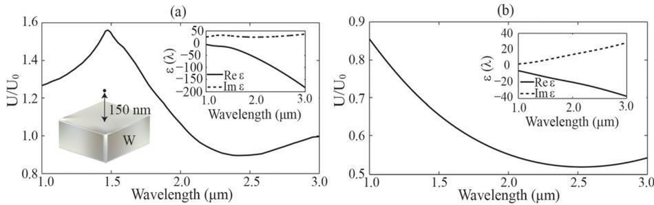
FIG. 1. (a) Near-field thermal emission normalized to the black-body emission ( $U_0$ ) for a 500 nm tungsten slab; the observation distance is 150 nm. (b) Normalized near-field thermal emission for a 500 nm TiN slab; same observation distance. The dielectric constants are shown in the inset. Such broadband near-field sources are not suited for thermophotovoltaics.
