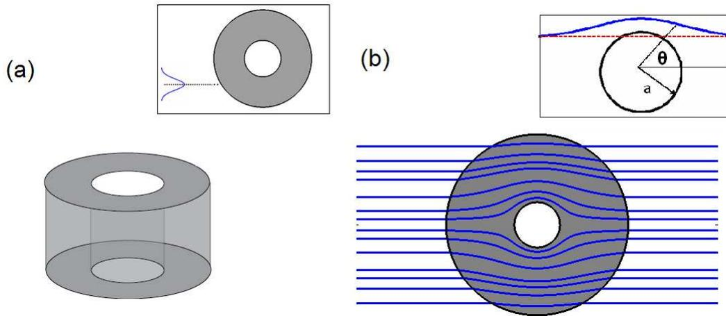
Fig. 1. (a) Cylindrical cloak, gaussian beam incident on the cloak (inset). (b) Calculated ray trajectories. Shown in the inset are ray trajectories in a cloaking medium (blue), ray trajectory in vacuum (red), cloaked region of radius  $a$
