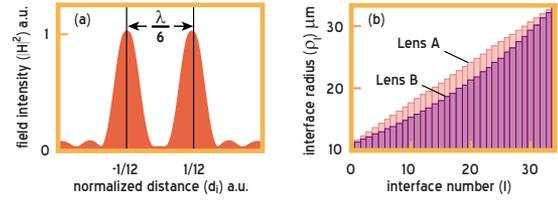
FIG. 2. (Color online) (a) Input magnetic field intensity at  $\rho_0$  used for all tests. (b) Comparison of the nonuniform distribution of  $\rho_{l_{\max}}$  obtained from Eq. (9) vs the uniform distribution;  $l_{\max} = 34$  has been taken for this example.
