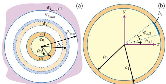
FIG. 1. (Color online) (a) Geometry of the concentric circular domains. (b) Example of the test source inside the zoomed internal region of the lens.
