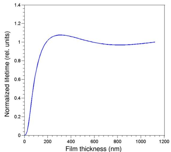
Fig. 4. (Color online) Calculated effective emission lifetimes of dipoles randomly oriented and uniformly distributed within PMMA film on the top of the silver-filled alumina membrane (normalized to the emission lifetime in pure PMMA).
