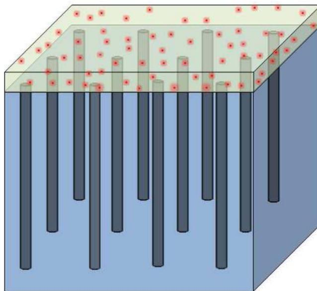
Fig. 1. (Color online) Schematic of the sample: alumina membrane with circular silver nanowires (a hyperbolic metamaterial) coated with dye-doped polymeric film.
