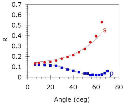
Fig. 2. (Color online) Angular dependence of the reflectance  $R$  in  $s$  and  $p$  polarizations at  $\lambda = 873$  nm. Solid lines—calculation according to Eq. (1) of [6].
